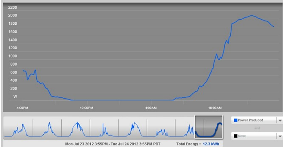
Figure 4.4. Solar PV system monitoring by Enphase: website.
