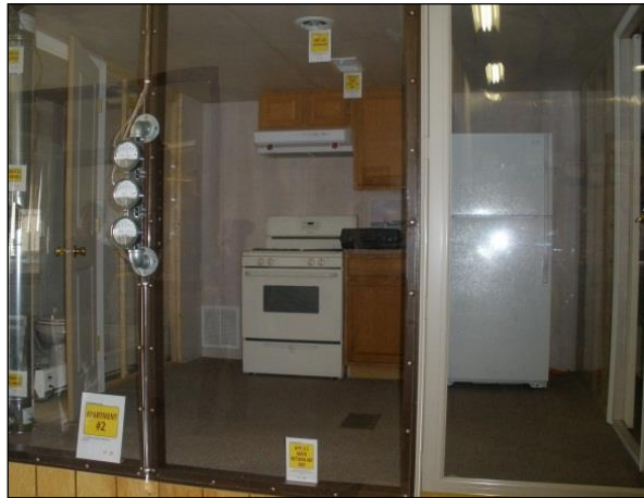
Fig. 13.5. At AEA's training facility, kitchen mock-up for CO testing on gas range and fridge metering
