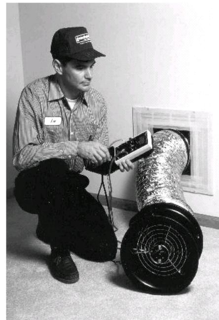
Figure 11.6. The Duct Blower (Photo courtesy of The Energy Conservatory).
