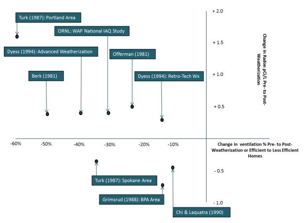
Figure 6. Findings Related to Change in Radon Levels as a Result of Change in Ventilation Pre- to Post-Weatherization for the ORNL Radon Study Compared to Relatable Studies
